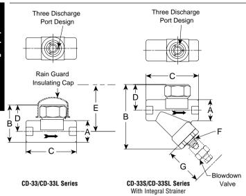
The Armstrong CD-33 is a disc style trap designed to control the trap's cycle rate. By reducing the cycle rate, the Armstrong CD-33 will have a longer service life than typical disc traps. This enhanced performance will ensure that maintenance time is minimized and steam costs are greatly reduced.
